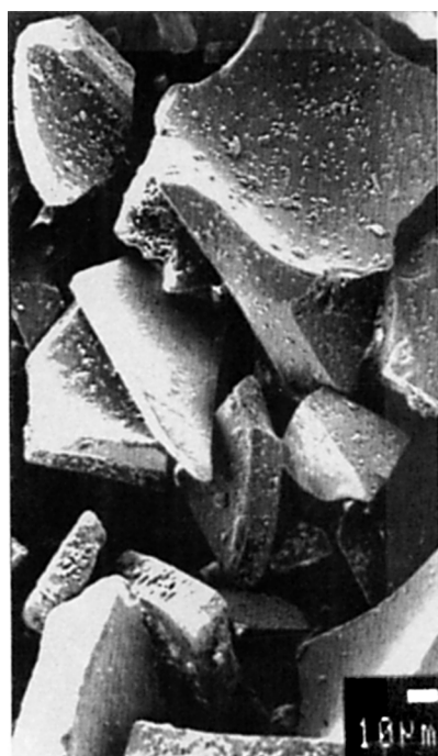
Figure 3 PBI powder particle morphology: (a) melt-derived powder, shardlike shape; (b) spray-precipitated powder, rounded shape.
